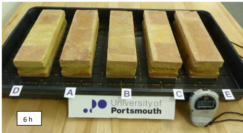
D – Conventional cream (Dryzone; A- Dryzone Rod Recipe 1; B Control (no treatment); C- Dryzone Rod Recipe 2; E- Low strength cream
